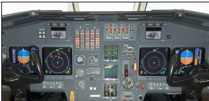
Photograph shows AVDU-1010 in pilot and co-pilot positions on Falcon jet for EVS application
